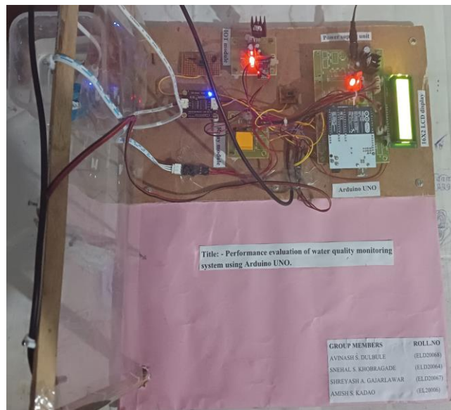
Fig.4. Model design for water quality monitoring system using Arduino UNO with IOT server based
