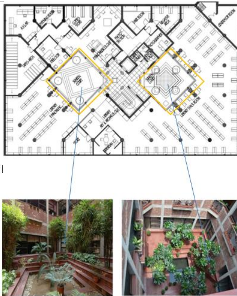
Figure 28 Position of sunken courtyard in American institute of Indian studies (Source: www.hrpub.org )
