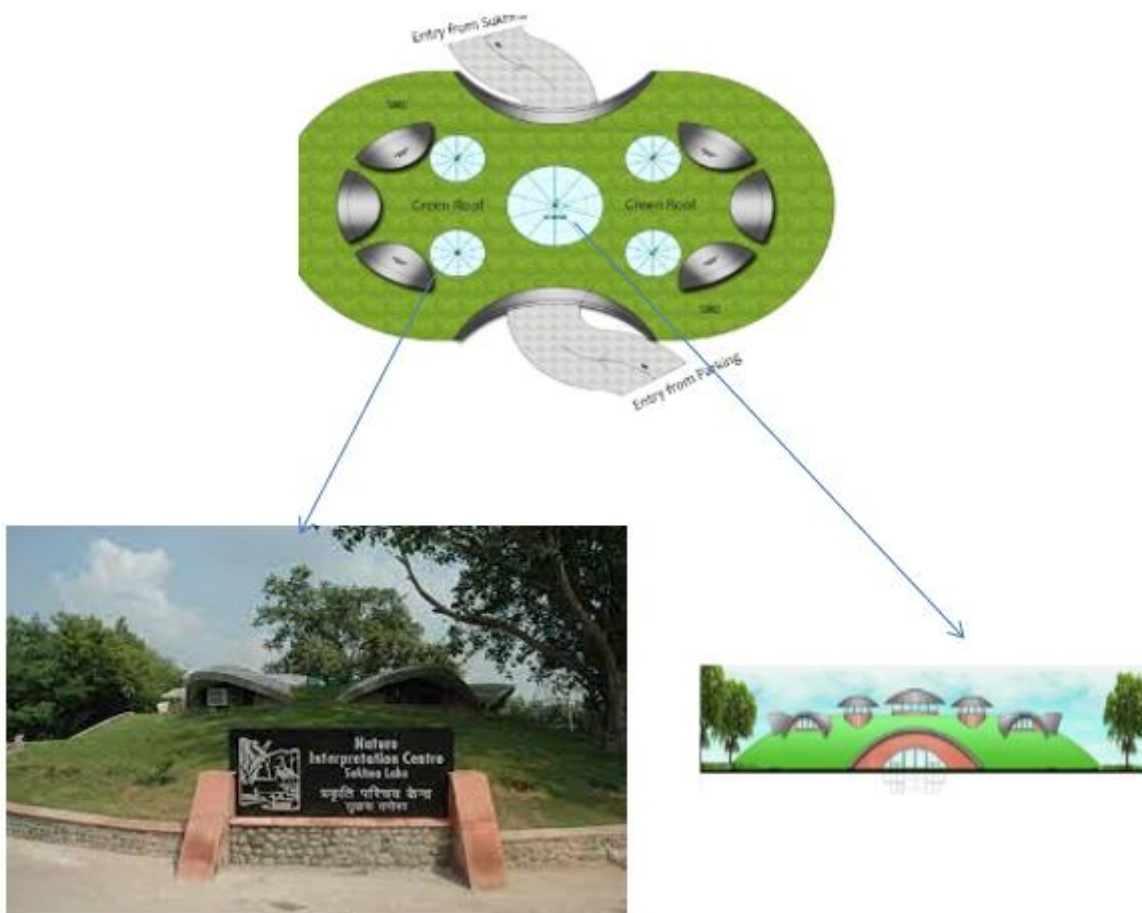
Figure 31 The position of skylight in nature interpretation center )Source: chandigarh.gov.in)
