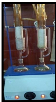
Fig 1 : Extraction in Soxlet apparatus
