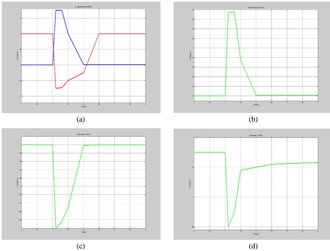
**Fig 13: Recovery of SREWH12T when storage node-pair Q-QB are affected by SEUs at VDD=1V
