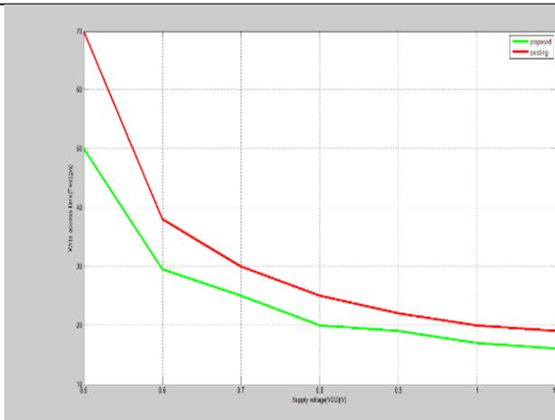
**Figure 6: TWA of all the considered cell at different VDDs**
