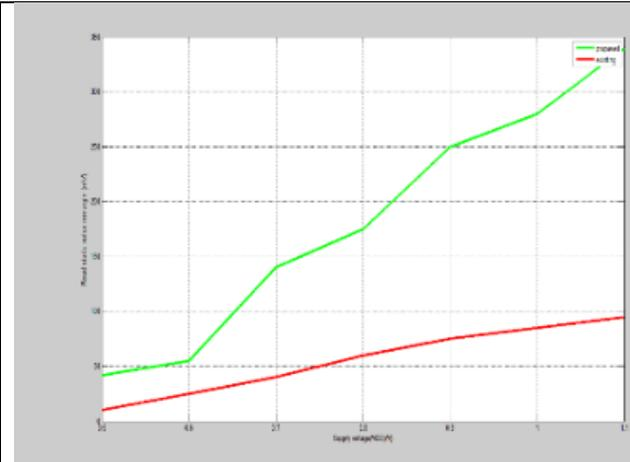
**Figure 5: RSNM of all the comparison cell at different VDDs.**
