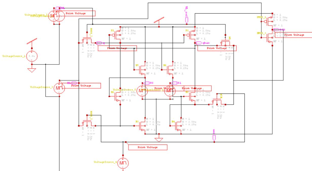
**Figure 1: Schematic of the SREWH12T SRAM cell.**
