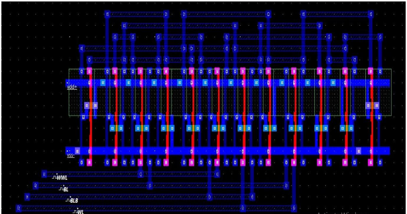
Figure 2: Thin cell Layout of SREWH12T SRAM cell.
