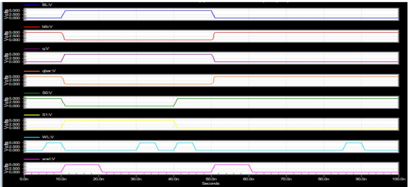
**Figure 3: Soft-error recovery at different nodes of the SREWH12T SRAM cell.**
