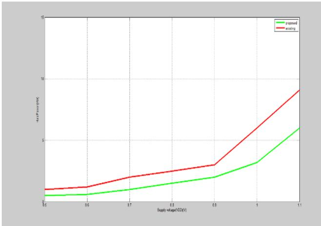
Figure 10: HPWR of all the considered cells at various VDDs.
