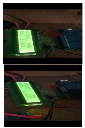
Whenever there is a short circuit, fire detection, or less voltage is been flowing through the system immediately we get the message in our app through Wi-Fi module also it specifies what the error is.
