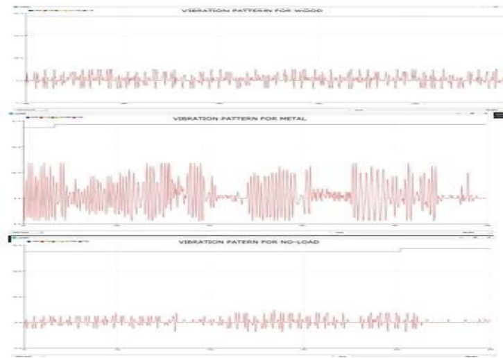
Fig.2. Accelerometer data during drilling activity
