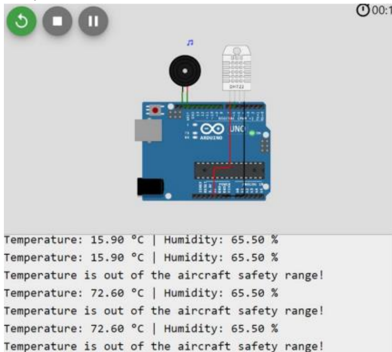
Fig. 4. Temperature & humidity sensor DHT22
