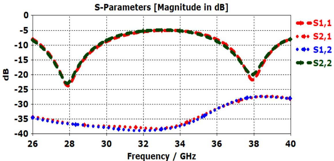
Fig 4. S-parameters of MIMO antenna.
