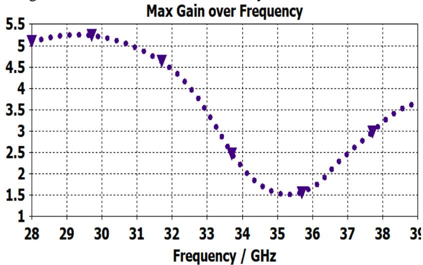
Fig. 10 The proposed antenna maximum gain
