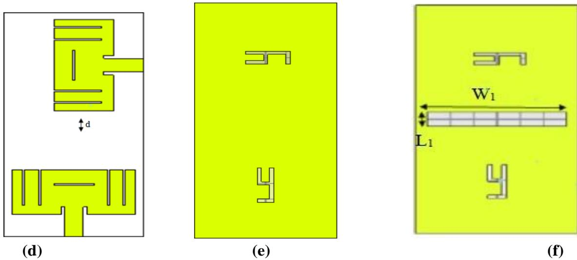
**Fig 1. The proposed MIMO antenna development stages: (a) Patch antenna, (b) Patch antenna with slots, (c) Ground with slots, (d) Proposed MIMO Geometry, (e) Ground without slot for isolation, and (f) Ground with slot for isolation.**
