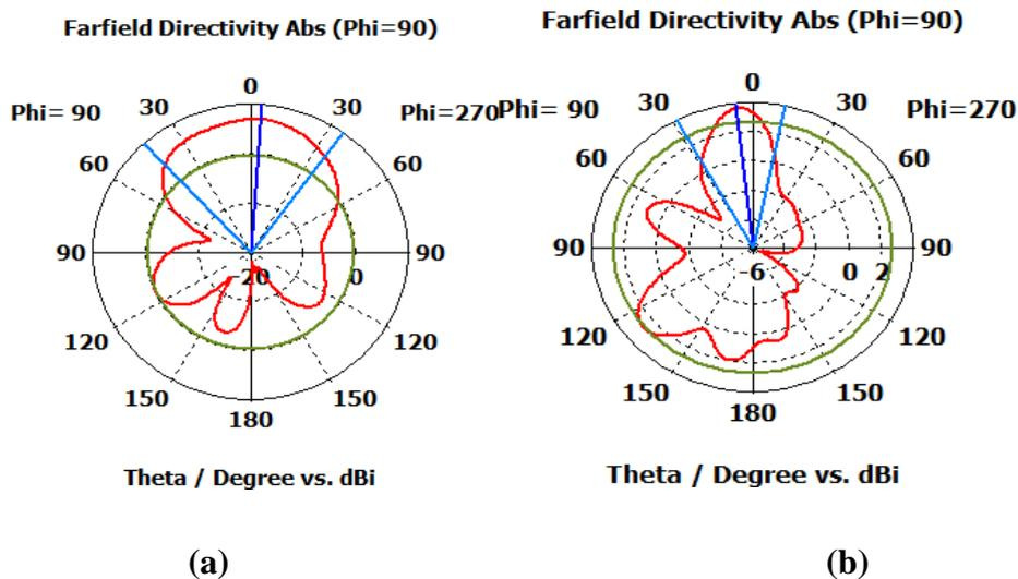
**Fig. 6 Radiation Pattern of port1 at (a) 28GHz and (b) 38GHz**
