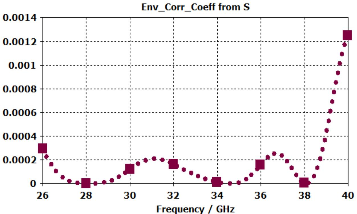
**Fig 8. Envelop correlation coefficient for MIMO antenna**
