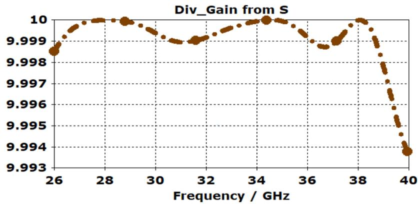
Fig. 9. Diversity Gain for MIMO antenna
