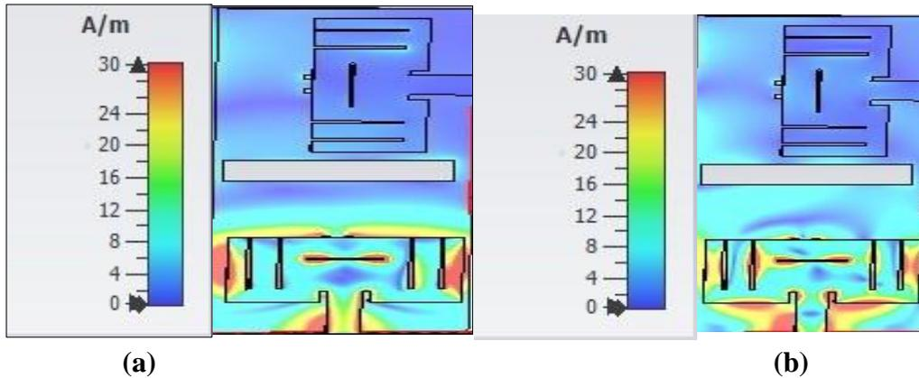
**Fig 5. Surface Current Distribution of port1 at (a) 28GHz and (b) 38GHz**
