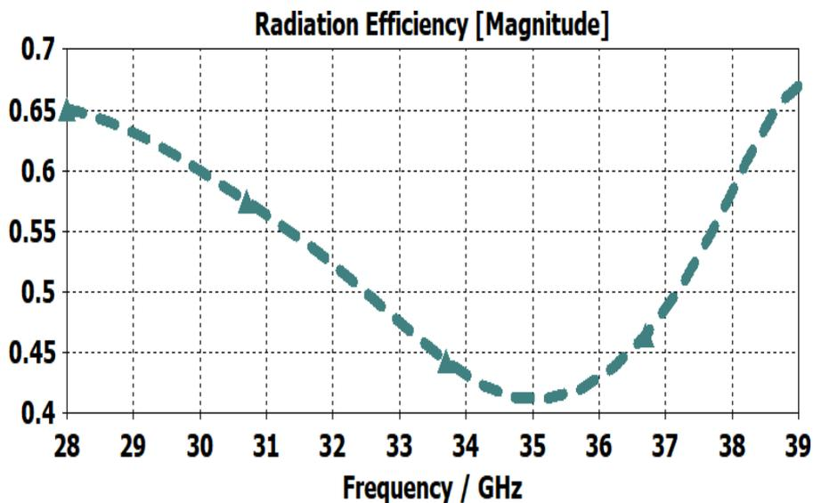
Fig 11. The proposed antenna radiation efficiency
