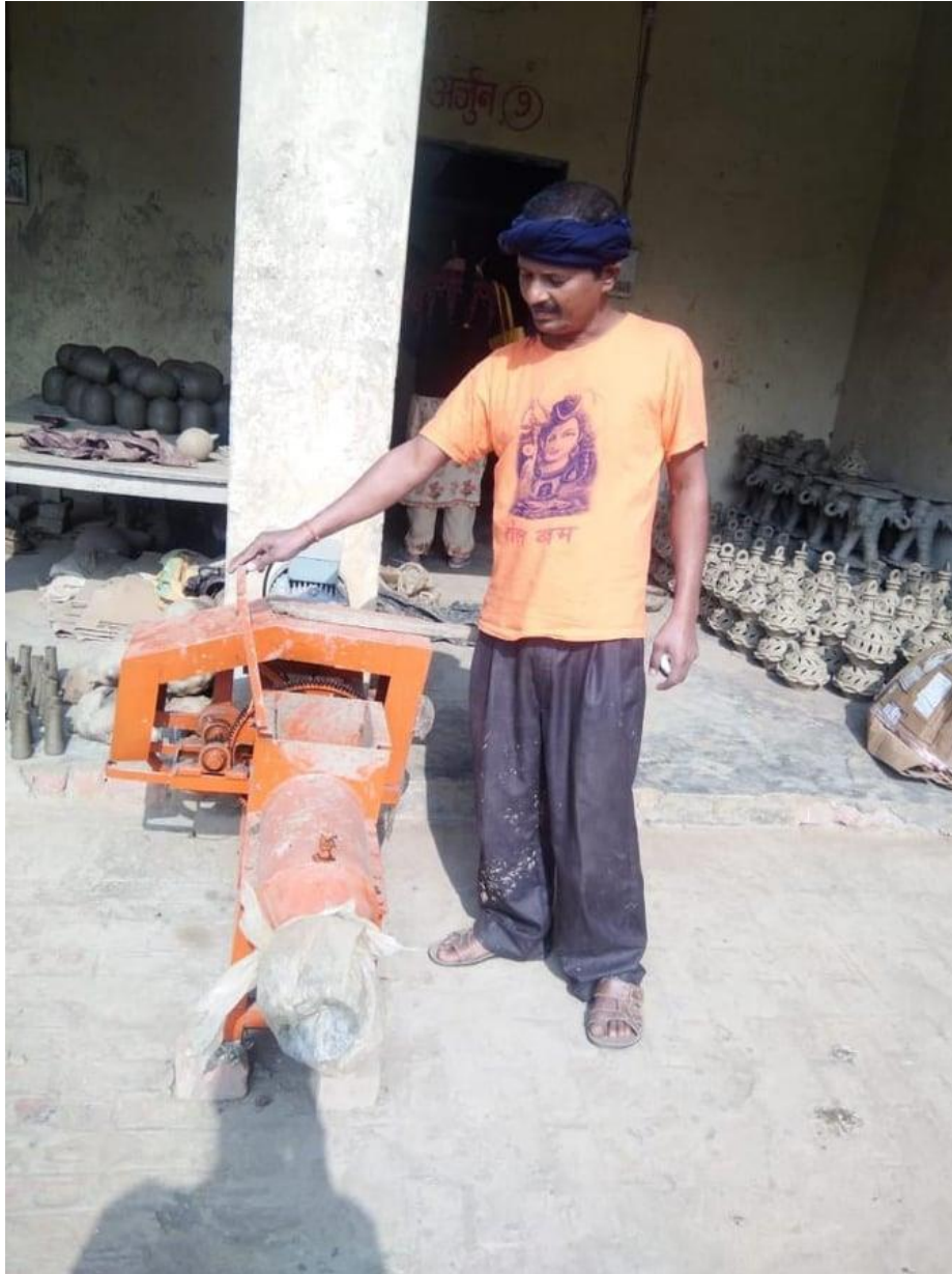
Fig.5. Machine used in refining clay
