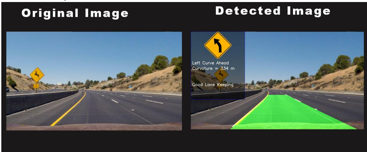
The Lane Line Detection Result
