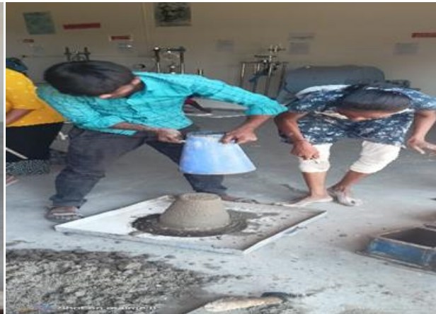
(b) slump cone test
