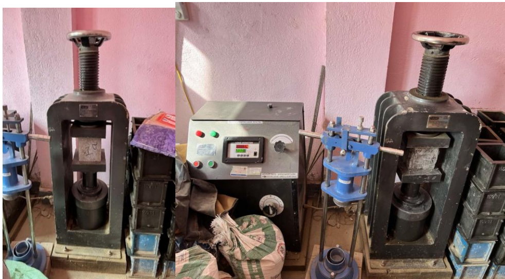
Figure 2: Determining compressive strength using a compression machine
