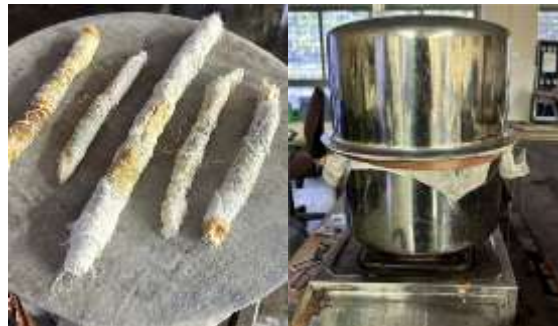
Figure 4: Fabric Bundles for Steaming after Tying
