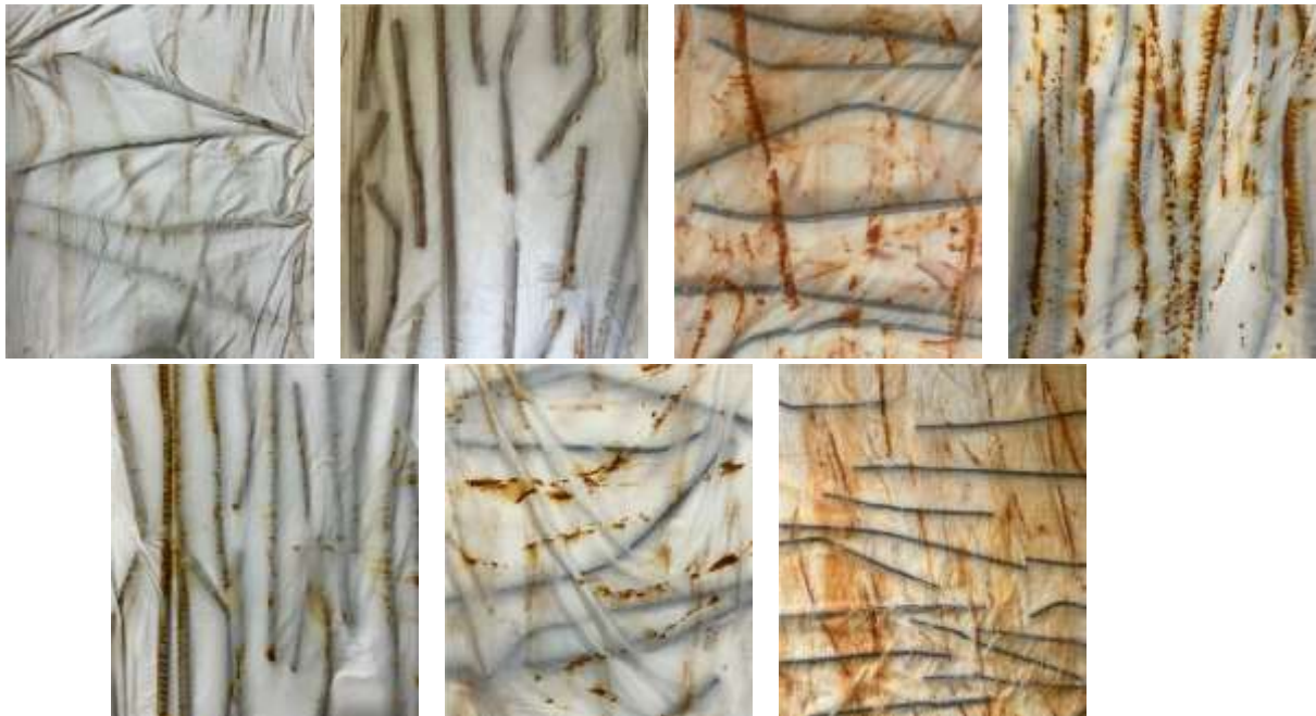
Figure 1: Rusted Iron Nails Placed on Wetted Cotton, Modal, Viscose and Polyester Fabrics
