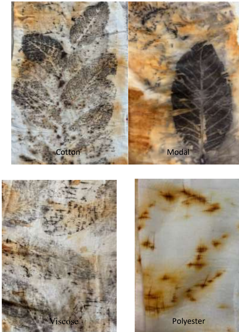
Figure 6: Results of Impressions Created by Mordant Applied Psidium guajava Leaves Over Rust Dyed Fabrics After Steaming Technique
