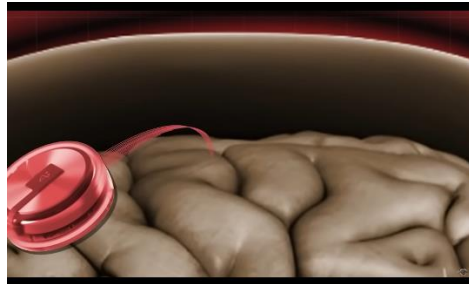
Fig 3.3: Neuralink N1 in Motor cortex
