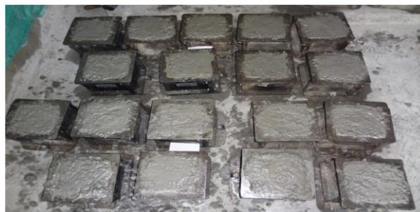
Figure 1: Concrete Casted in Moulds
