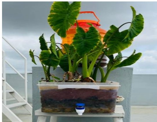
Fig 2: Setup of artificial vertical subsurface flow wetland model using the C. esculenta plant
