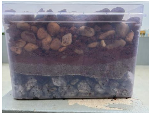
Fig 1: Materials setup in Vertical subsurface flow artificial wetland model
