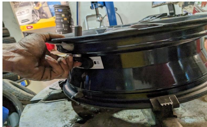
Fig 7. Sensors mounted on vehicle wheel
