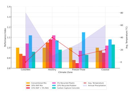
Performance index values above 1.0 indicate improvement over conventional mix. Note the superior performance of recycled rubber in freeze-thaw conditions and recycled plastic in hot/dry environments. Data collected from test sections in 12 states over a 24-month evaluation period (2022-2023). *Performance Index: Ratio of material performance compared to conventional mix (higher is better)*
