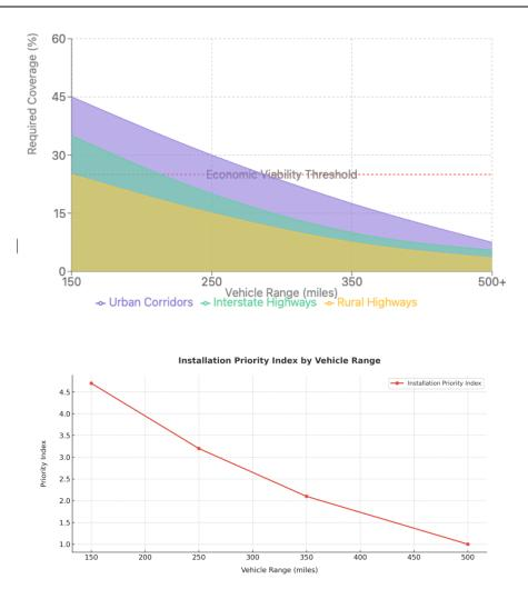
Analysis of required wireless charging infrastructure coverage based on vehicle range capabilities. As vehicle range increases, the required charging infrastructure density decreases substantially, particularly in rural areas. Installation priority index reflects the relative urgency of deployment based on current EV market penetration and range anxiety factors. Data derived from U.S. Department of Transportation modeling and industry projections (2024).
