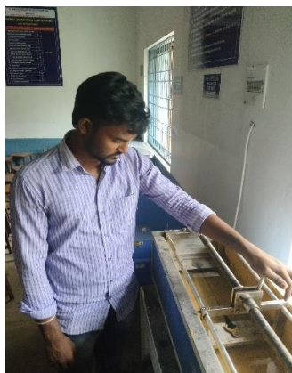
Fig (5) Bitumen Ductility Test
