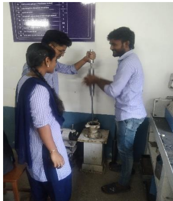
Fig (6) Cube casting
