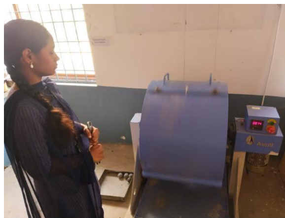
Fig (4) LA Abrasion test for Hardness
