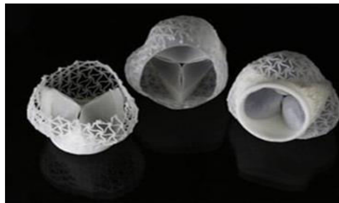
Figure 2: Printed Heart valve replacement systems with leaflets and synthetic aortic root [12].
