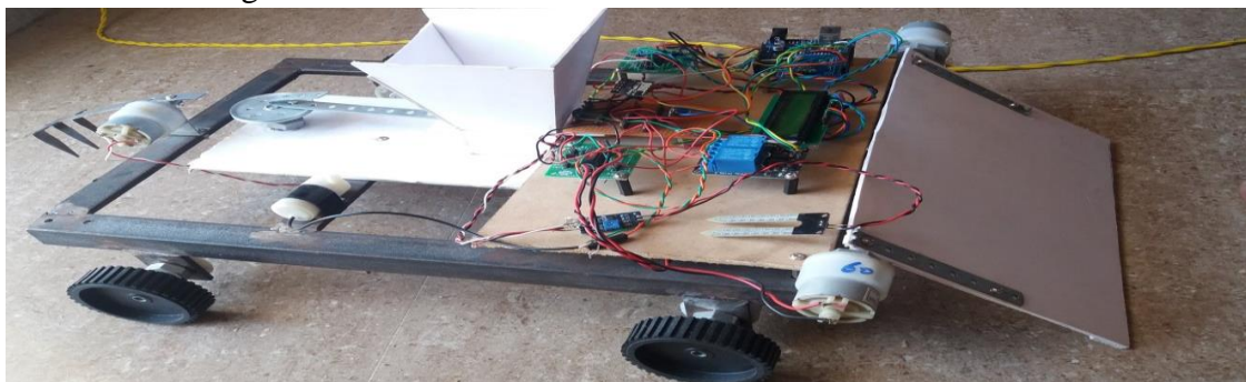
FIG 3 MODEL OF MULTI-PURPOSE AGRO-ROBOT
