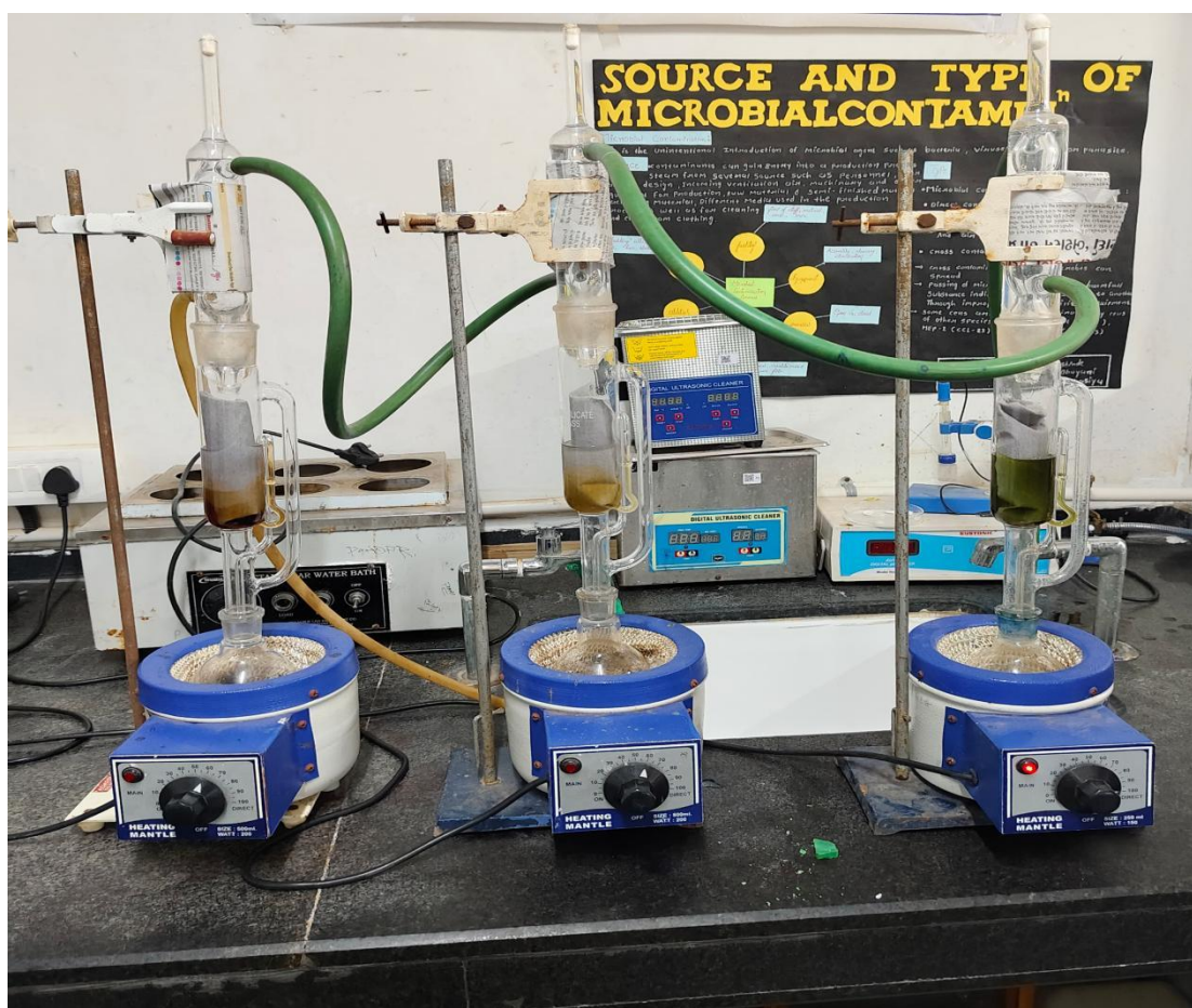
[Figure 12: Soxhlet Apparatus Setup for Extraction]
