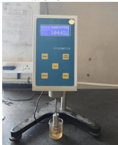
[Figure 16: Viscosity Measurement]
