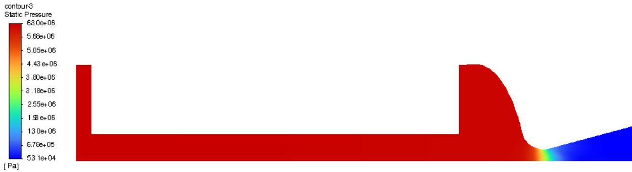
Figure 7: Contour of static pressure showing the pressure drop at the throat
