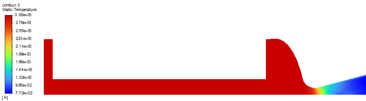
Figure 8: Contour showing decreasing of temperature at the outlet
