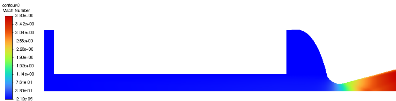
Figure 6: Contour of Mach number showing change of flow from subsonic to supersonic.
