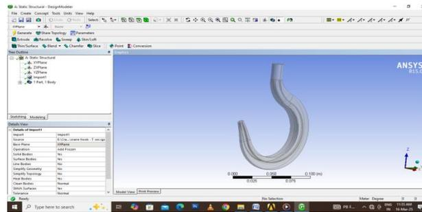
Fig 4.2 The catia model of crane hook is imported to Ansys 15.0
