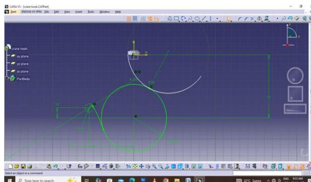
Fig 3.1 Basic sketch of the profile of crane Hook in Catia V5
