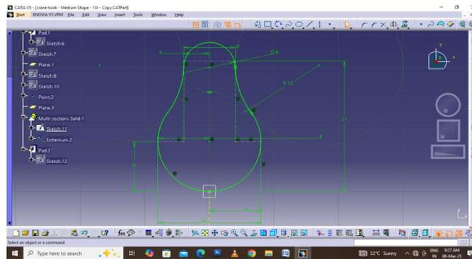
**Fig 3.6 Basic sketch of intermediate shape of crane hook**
