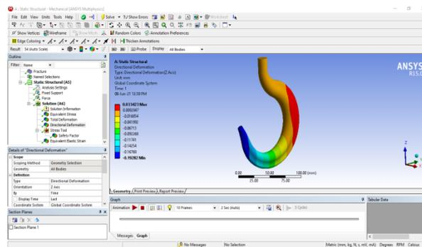
Fig 5.14 Total deformation development in Crane Hook Model-5
