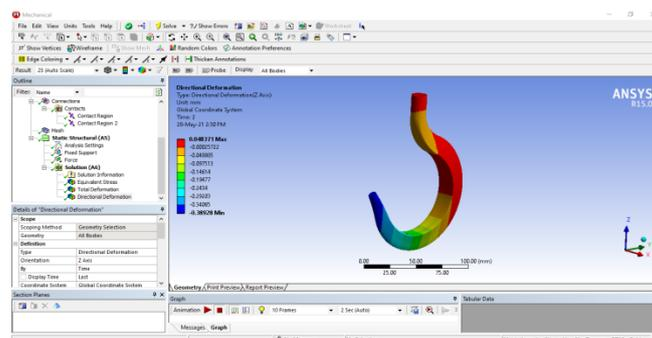
**Fig 5.2 Total deformation development in Crane Hook with Trapezoid cross section: Model-1**
