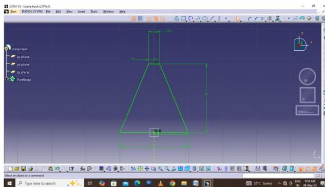
**Fig 3.3 The sketch of cross section of the crane hook in Catia V5**
