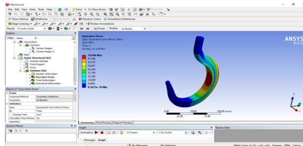
**Fig 5.1(b) Equivalent Von-mises Stress distribution in Crane Hook with Trapezoid cross section: Model-1(other view)**
