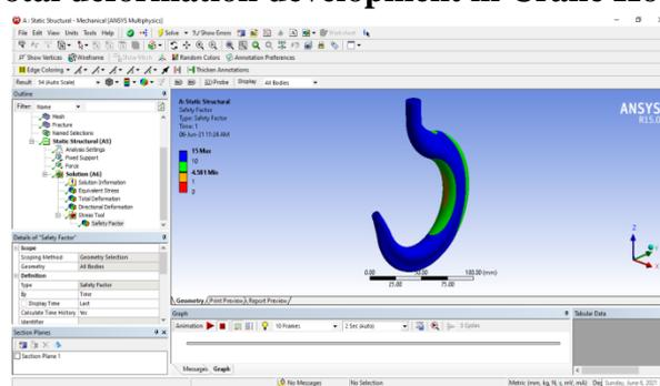
Fig 5.15 Safety Factor attained in Crane Hook Model-5
