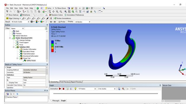
**Fig 5.18 Safety Factor attained in Crane Hook Model-6**
