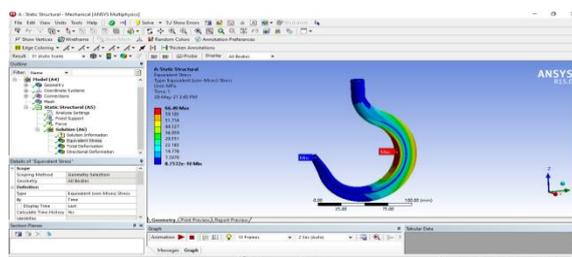
**Fig 5.4(a) Equivalent Von-mises Stress distribution in Crane Hook with “T” cross section: Model-1**
