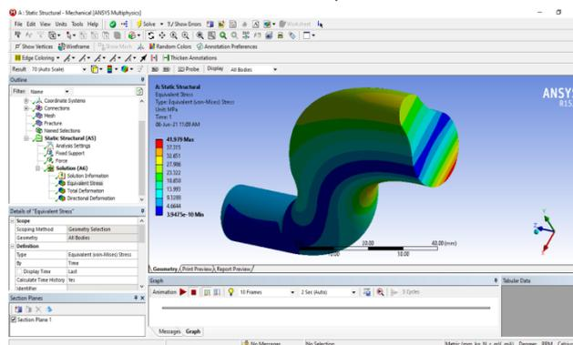
**Fig 5.10(b) Equivalent von-mises Stress distribution in Crane Hook Model-4 (Cross sectional view at highly stressed section)**
