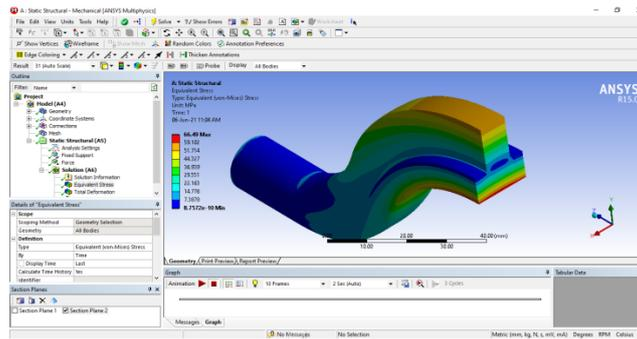
**Fig 5.4(b) Equivalent Von-mises Stress distribution in Crane Hook Model-2 (Cross section view at highly stressed section)**
