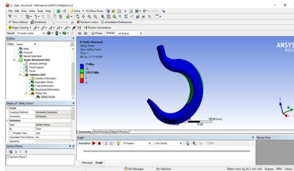
**Fig 5.12 Safety Factor attained in Crane Hook Model-4**
