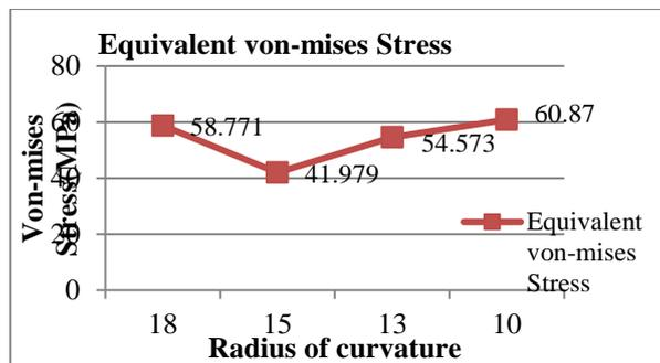
Fig 5.19 Effect of radius of curvature on the von-mises stress development
