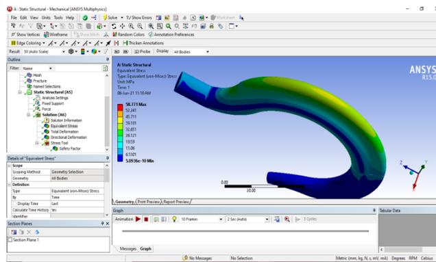
Fig 5.7(b) Equivalent von-mises Stress distribution in Crane Hook Model-3 (other view)
