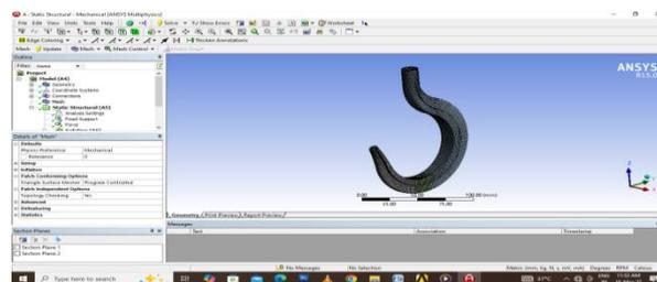
Fig 4.4 Meshed model of Crane Hook in Ansys 15.0
