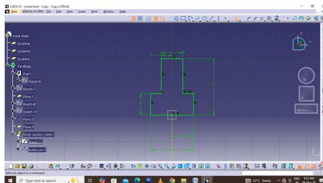
**Fig 3.5 Basic sketch of T shape cross section of crane Hook in Catia V5**
