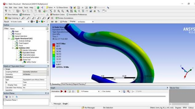
Fig 5.13(b) Equivalent von-mises Stress distribution in Crane Hook Model-5 (other view)
