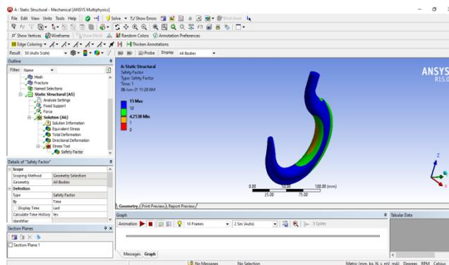
Fig 5.9 Safety Factor attained in Crane Hook Model-3
