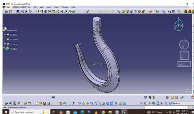
**Fig 3.4 The created model of Crane hook model with trapezoid cross section in Catia V5**
