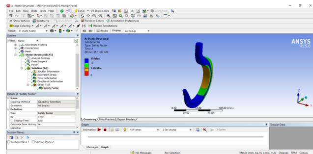
**Fig 5.6 Safety Factor attained in Crane Hook with T-cross section: Model-2**
