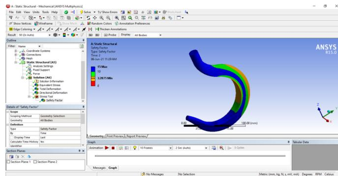
**Fig 5.3 Safety Factor attained in Crane Hook with Trapezoid cross section: Model-1**
