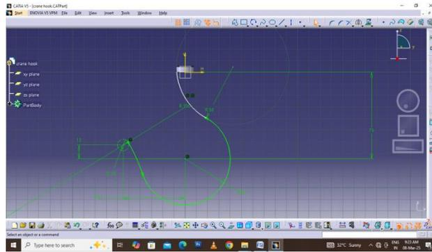
**Fig 3.2 The complete profile of considered crane hook in Catia V5**
