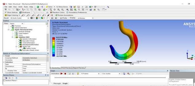
**Fig 5.17 Total deformation development in Crane Hook Model-6**
