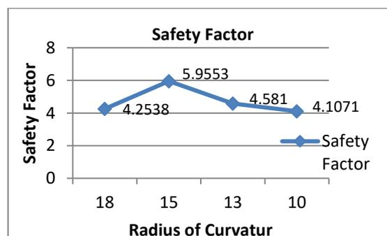
Fig 5.21 Effect of radius of curvature on the critical safety factor
