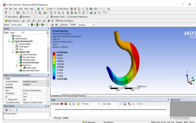
Fig 5.8 Total deformation development in Crane Hook Model-3
