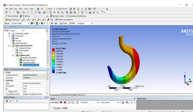
**Fig 5.11 Total deformation development in Crane Hook Model-4**
