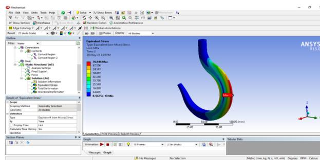
**Fig 5.1(a) Equivalent Von-mises Stress distribution in Crane Hook with Trapezoid cross section: Model-1**
