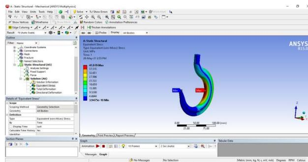
**Fig 5.10(a) Equivalent von-mises Stress distribution in Crane Hook Model-4 (Intermediate Cross section)**
