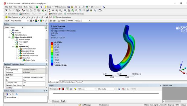
**Fig 5.16(a) Equivalent von-mises Stress distribution in Crane Hook Model-6 (Intermediate Cross section)**
