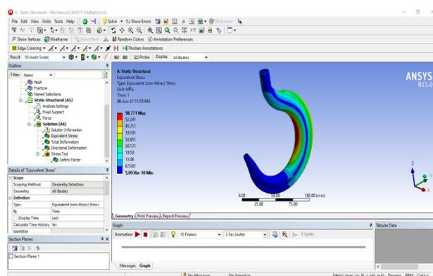
**Fig 5.7(a) Equivalent Von-mises Stress distribution in Crane Hook Model-3 (Intermediate Cross section)**
