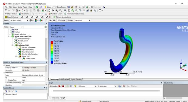
**Fig 5.13(a) Equivalent von-mises Stress distribution in Crane Hook Model-5 (Intermediate Cross section)**
