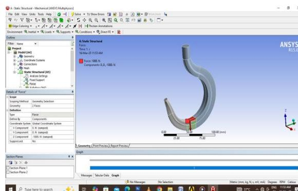
Fig 4.6 Applying load to the model.
