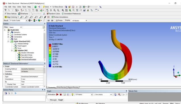
**Fig 5.5 Total deformation development in Crane Hook with T- cross section: Model-2**
