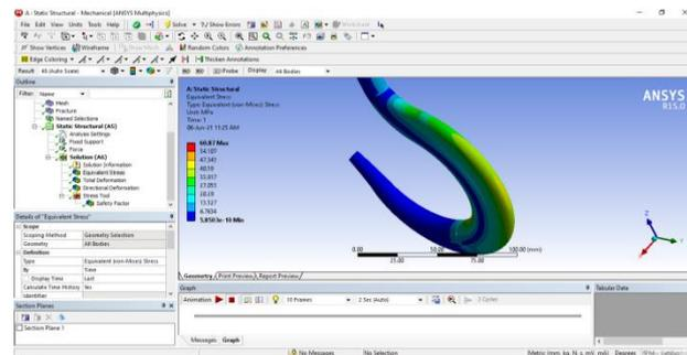
**Fig 5.16(b) Equivalent von-mises Stress distribution in Crane Hook Model-6 (other view)**
