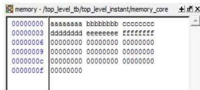
Fig. 6: Memory flash core is initialized with random data
