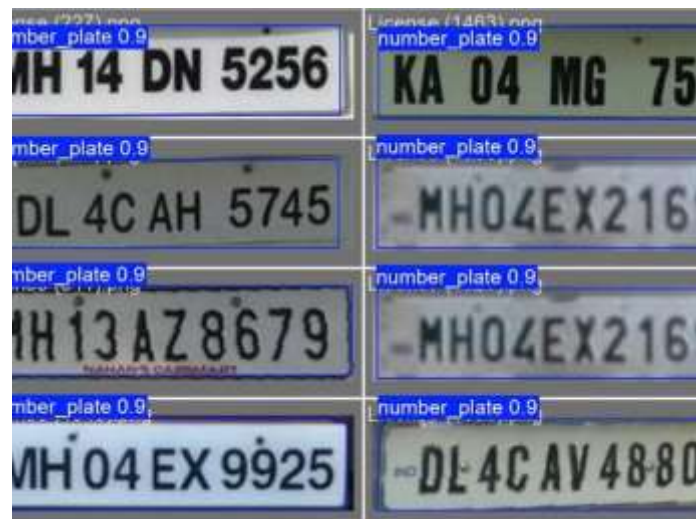
Figure 8: Sample image showing annotated number plate extracted using OpenCV and YOLOv8 detection
