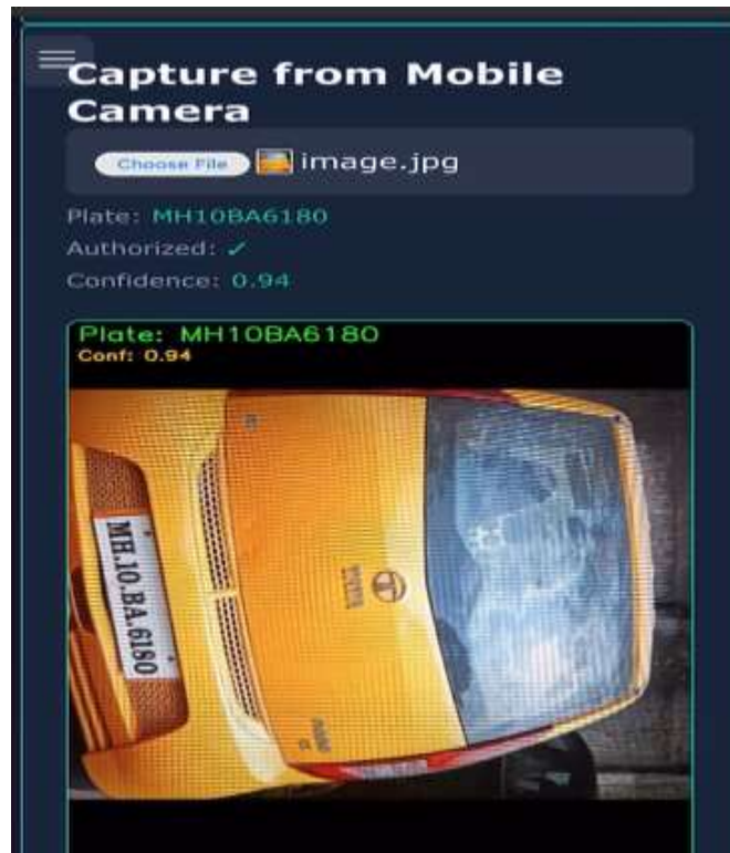
Figure 11: System detects a match - vehicle marked as ‘Authorized’ and granted entry.
