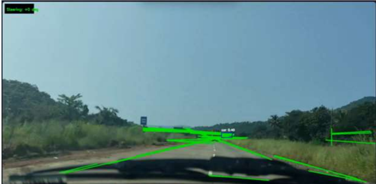
Figure 3: Pothole detected within the lane with calculated deceleration value.
