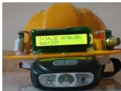
Figure 13: Outlook of smart helmet and LCD Displaying Temperature, Humidity and Gas Measurement Values.
