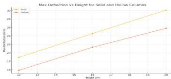
Here's a sample chart comparing Max Deflection vs Height for Solid and Hollow columns. This gives a clear visual distinction between the two types.
