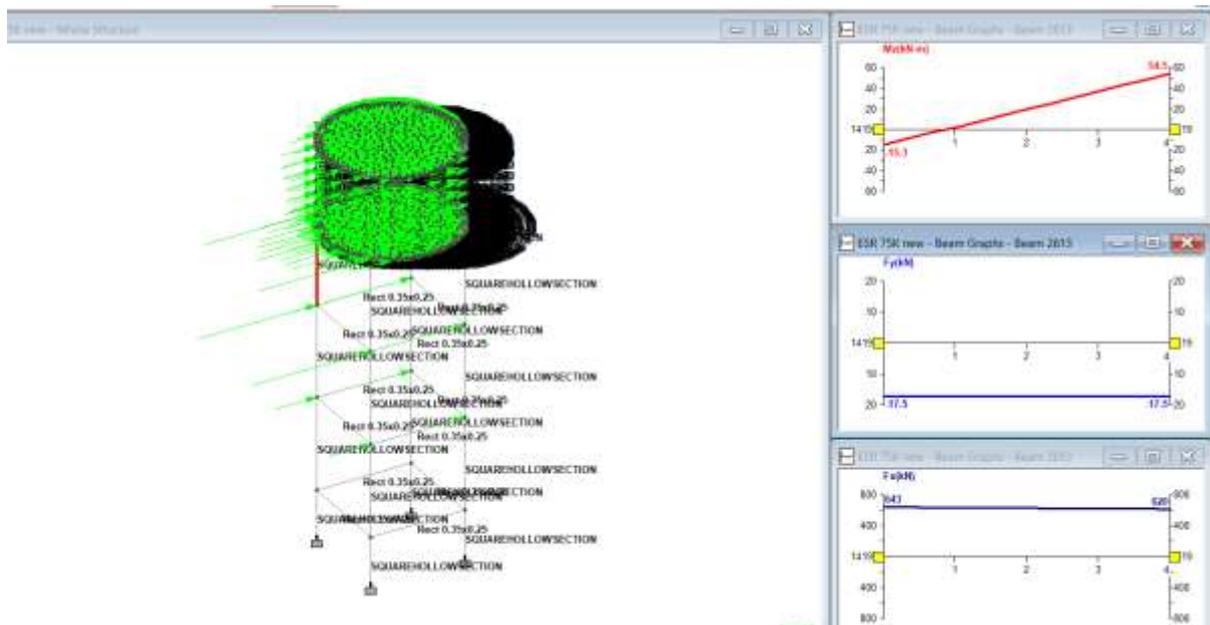
Fig. 3.2 EQ forces , BMD and SF of of water tank of hollow column 12 m staging
