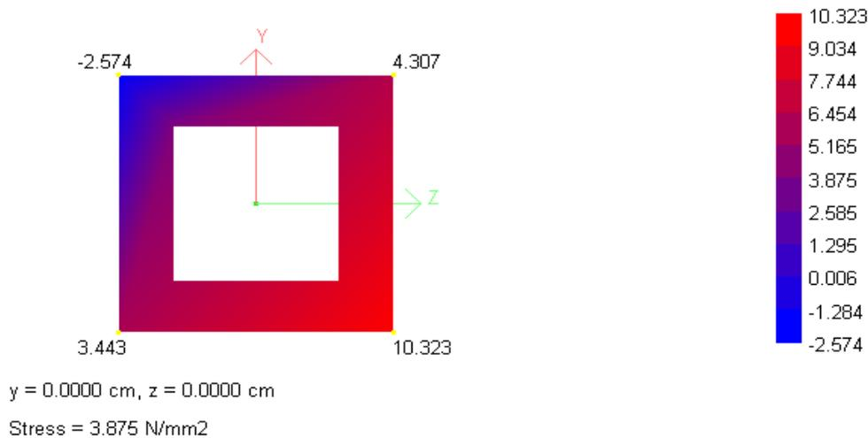
**Fig. 4.4 Bending stresses in column water tank of hollow column 12 m staging**
