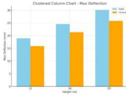
**Fig. 4.2 Staging height wise Comparison of max deflection v/s height of solid and hollow column**
