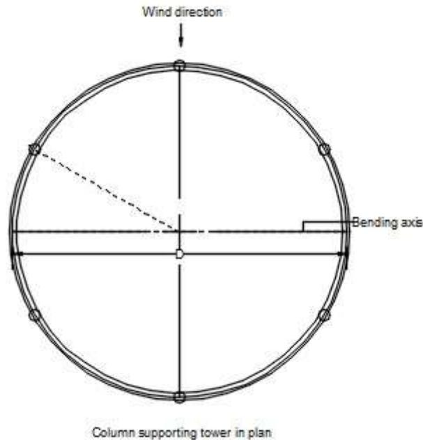
**Fig. 1.2 Column of supporting tower in plan**
