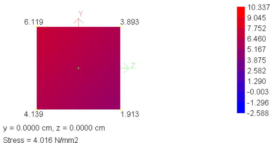
**Fig. 4.5 Bending stresses in column water tank of solid column 12 m staging**
