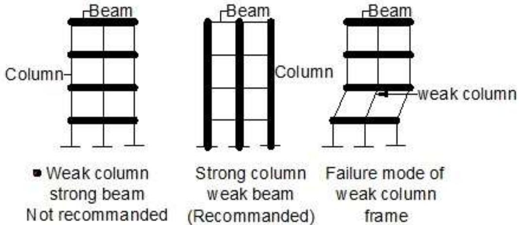
Fig. 1.3 Weak beam-strong column concept
