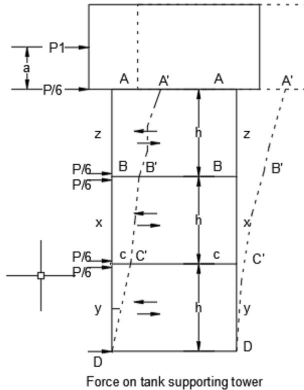
**Fig. 1.1 Forces on tank supporting tower**
