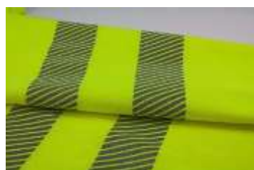
Figure 29: Antistatic+flamer-etardent combination fabric
