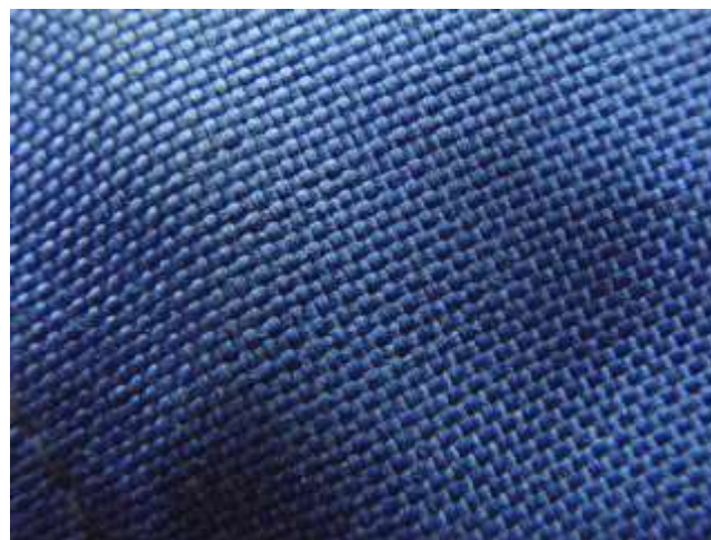
Figure 14: Close-up of a ballistic nylon 2 x 2 basket weave
