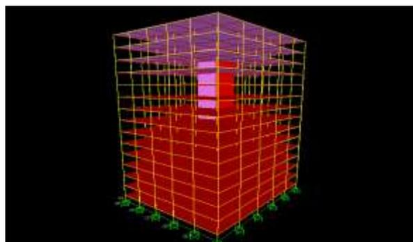
**Fig.4.2: 3D View Line Type Shear Walls at Centre of the Building**
