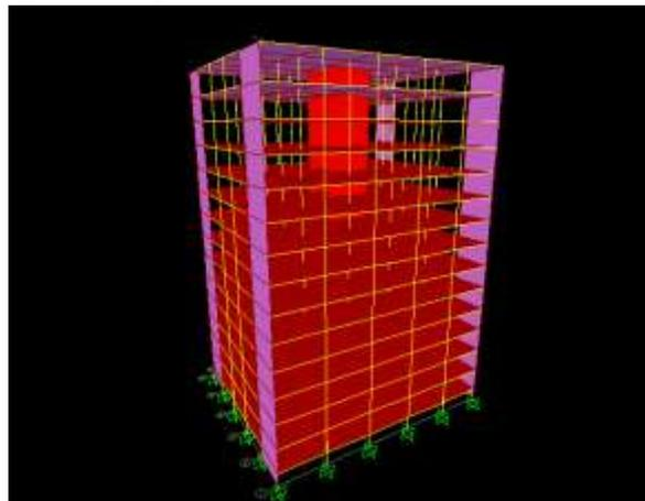
**Fig.4.2: shear walls at side ends and middle of the building**
