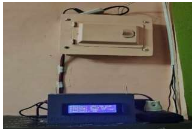
Figure 4.1 Fully Integrated Setup of the Real-Time Energy Monitoring System with the Main Panel Board
