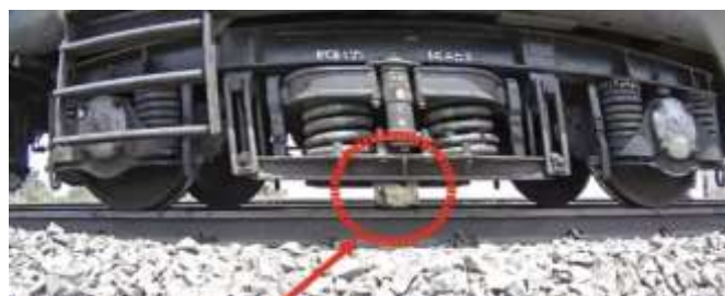
Fig: 7 Hanging part detection
