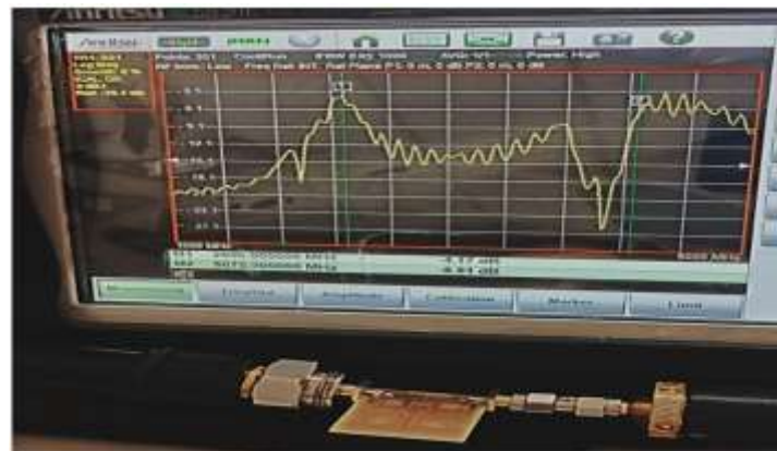
Figure 10. Snapshot of fabricated filter tested with network analyzer
