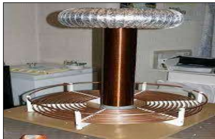
Figure 4. Typical loosely coupled design
