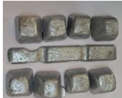
Fig 1.1 Casted billets of LM26
