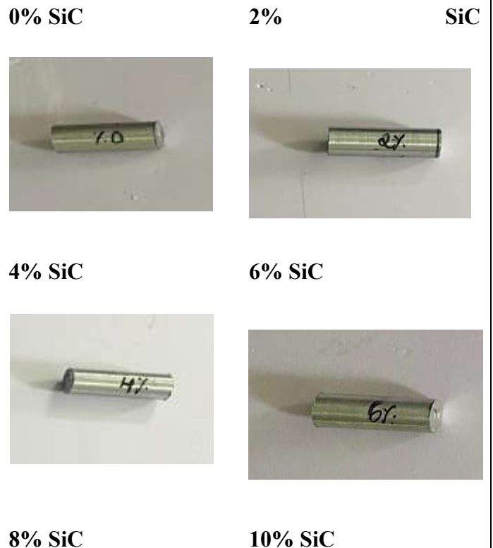
Fig 3.2 Pin on disc test specimen as per ASTM standard with varying percentage of SiC
