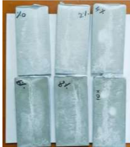
Fig 2.2 Casted MMC's for varying SiC% plates.
