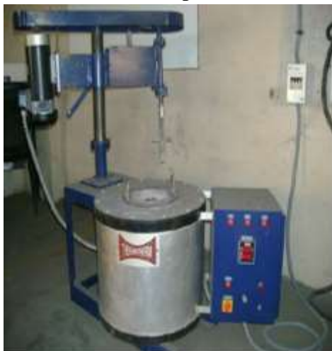
Fig 2.1 Electrical power operated, Temperature control Stirring mechanism casting machine setup
