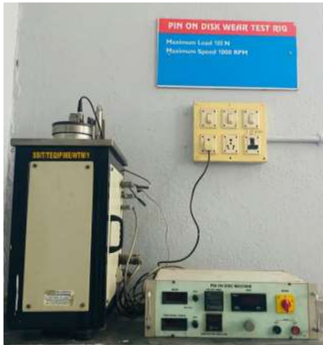
Fig 3.1 Pin on disc wear test setup
