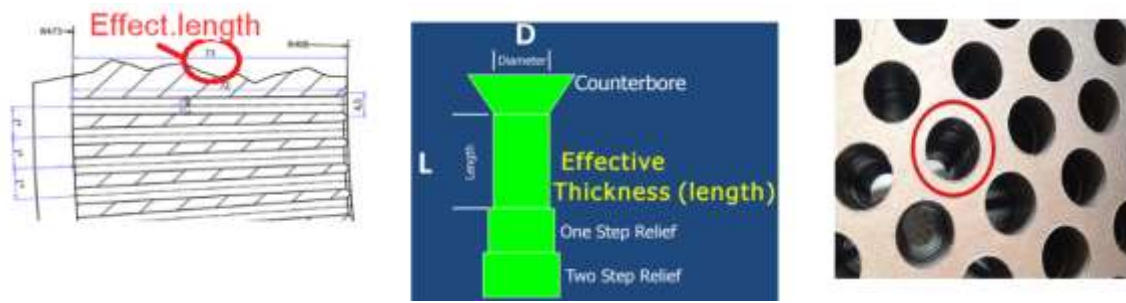
Figure 2.3: Pellet press disc effective size and shape, internal structure of the matrix
