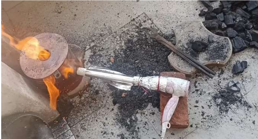
Figure 2: Coal-fueled blacksmith furnace used for paste-based surface hardening at \sim 950^{\circ}\text{C} .
