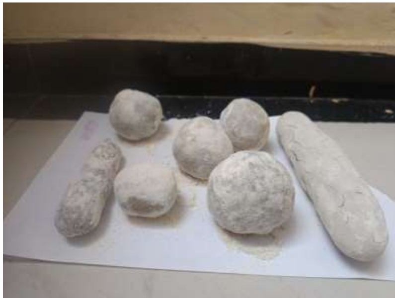
Figure 1: Mild steel specimen coated with organic paste and sealed with clay before heat treatment.
