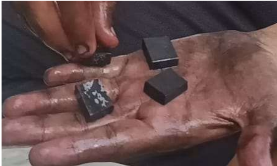
Figure 3: Specimen after paste carbonitriding treatment (Charcoal + Urea + Eggshell).
