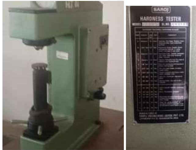
Figure 5: Rockwell hardness testing machine (Model RAB1, S.No SN5421) used for hardness evaluation.
