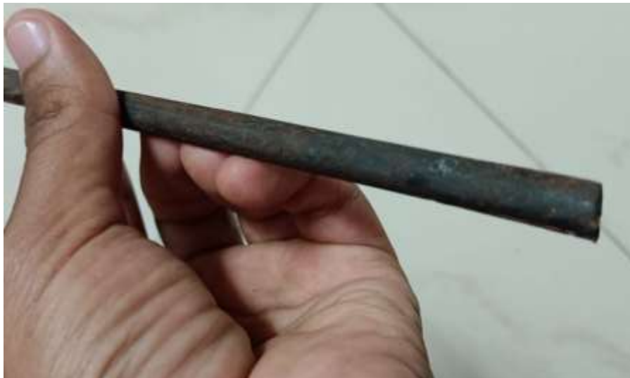
Figure 4: Specimen after paste carburizing treatment (Charcoal + Salt).
