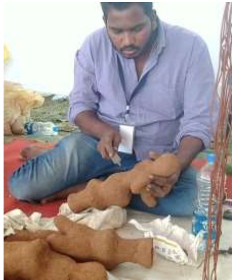
Figure 11. Iron nails are added as core pins
