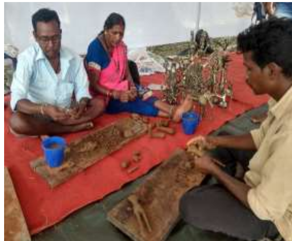
Figure 3. Creating core body with clay.
