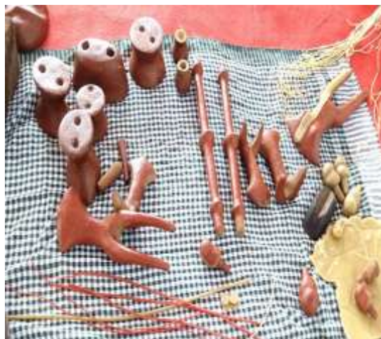
Figure 4. Wax layer is applied on sundried clay core body.
