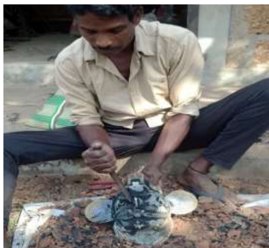
Figure 22. Chisels are used to remove the mould remains.
