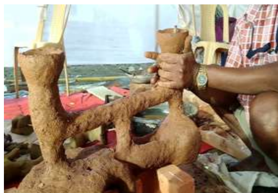
Figure 10. Clay funnel is attached with wax runner on the mould
