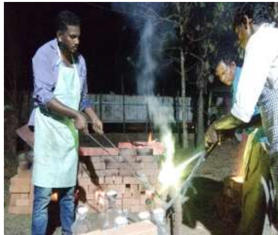
Figure 20. Pouring molten metal into the moulds
