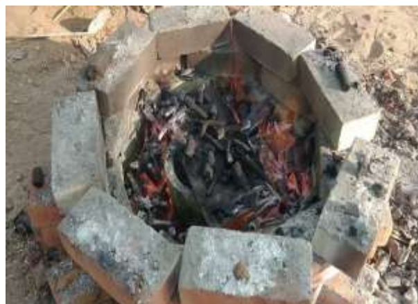
Figure 19. Traditional furnace with coal firing
