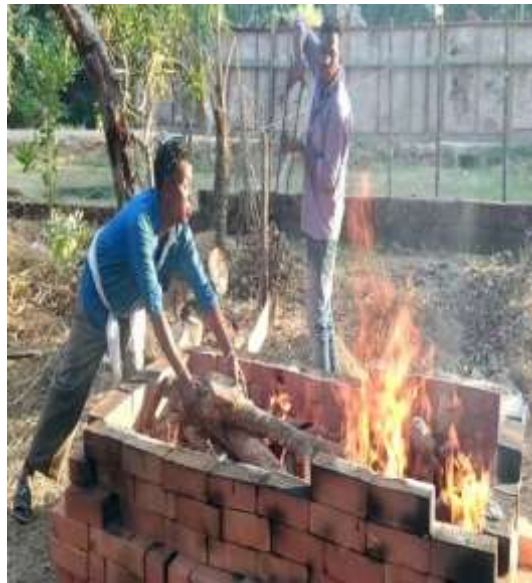
Figure 17. Dewaxing process of moulds in local kiln
