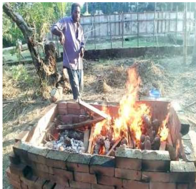
Figure 18. Iron tongs are used to add woods gently around the moulds
