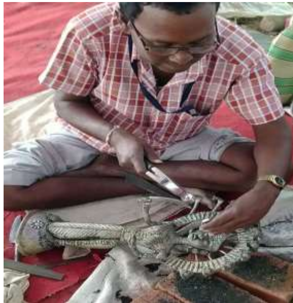
Figure 23. Nails are removed from the cast with chisel
