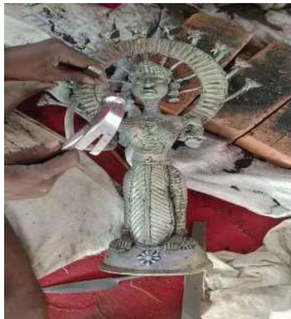
Figure 24. Unwanted metal flashes are chiselled carefully
