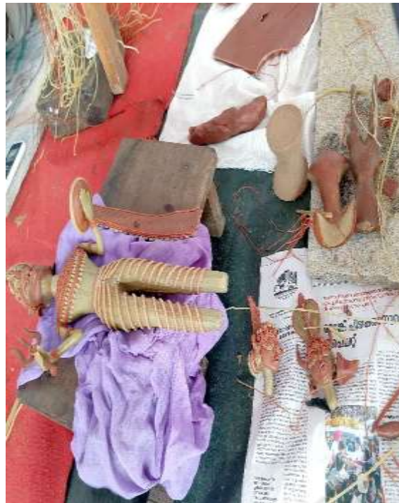
Figure 6. The wax model is kept on piece of cloth, to assemble the parts
