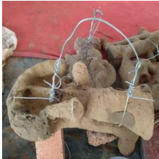
Figure 15. Handle is created with galvanised wire on large size moulds
