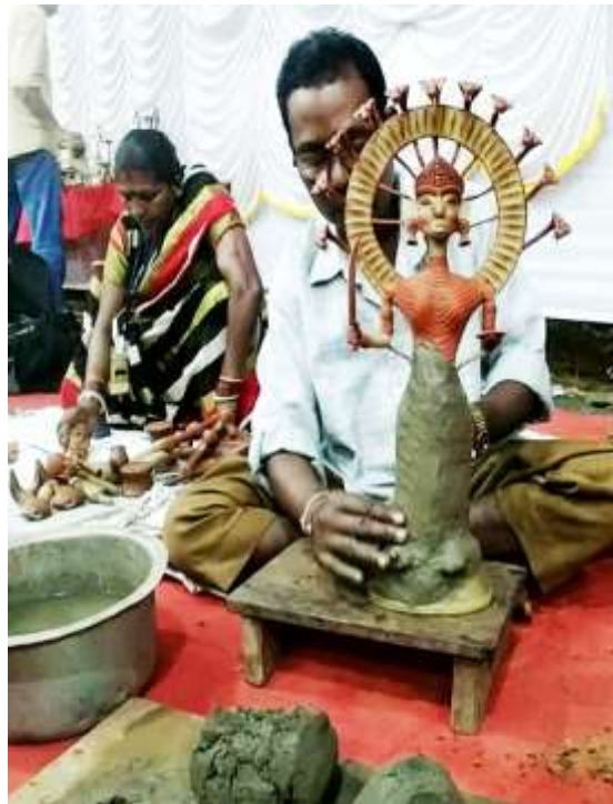
8. First layer of fine clay is applied for mould making process.
