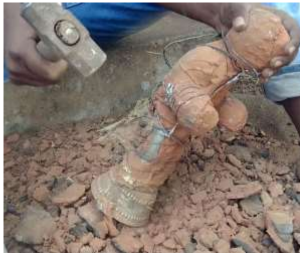
Figure 21. The mould is removed from the cast with a hammer.
