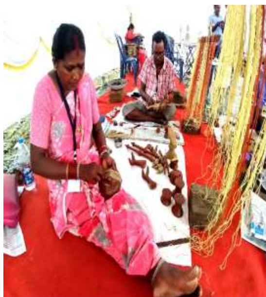
Figure 5. Modelling with wax strings on core body.
