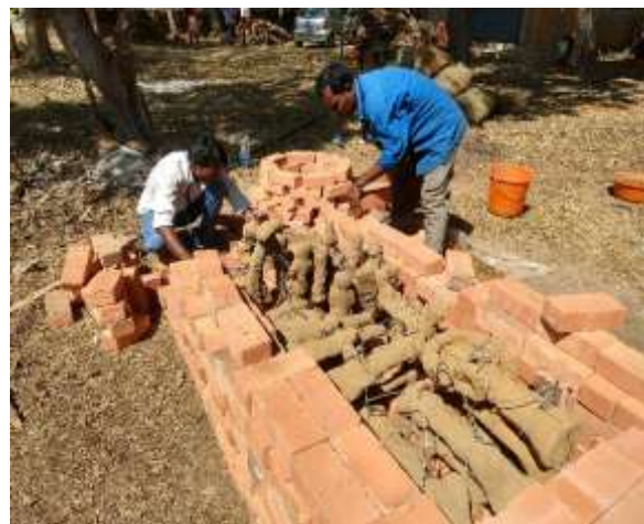
Figure 16. Local kilns are prepared with bricks
