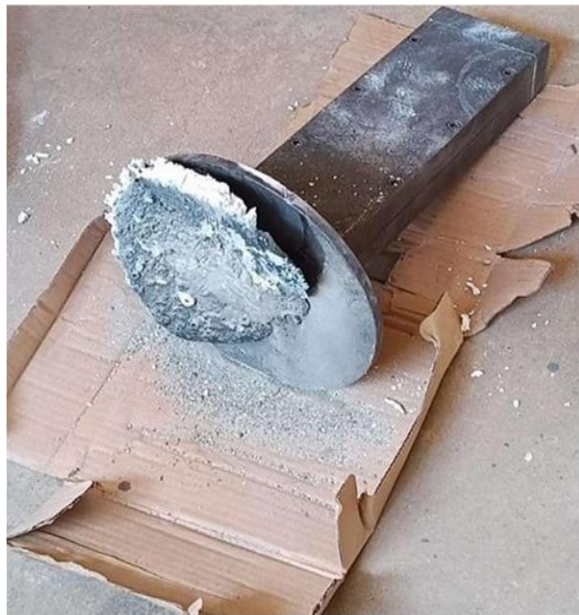
Fig.6.7 Casted magnesium rod
