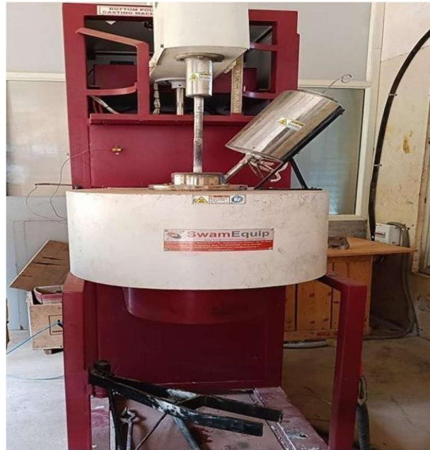
Fig.6.1 Laboratory stir casting setup
