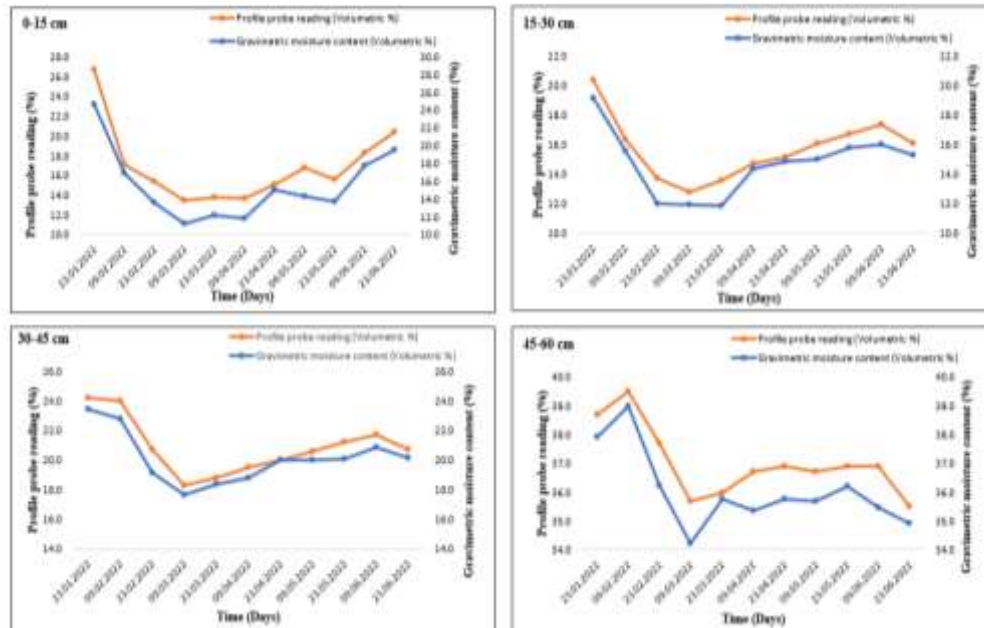
Fig.1: Comparison of moisture content (%) measured using Profile probe and gravimetric method in 4 depths with respect to time (days)
