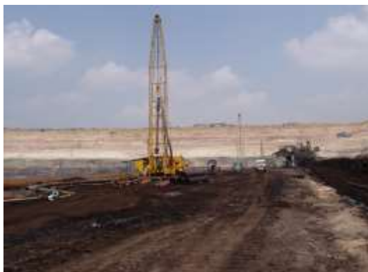
Reverse circulatory drill positioned for drilling large diameter well for depressurization
