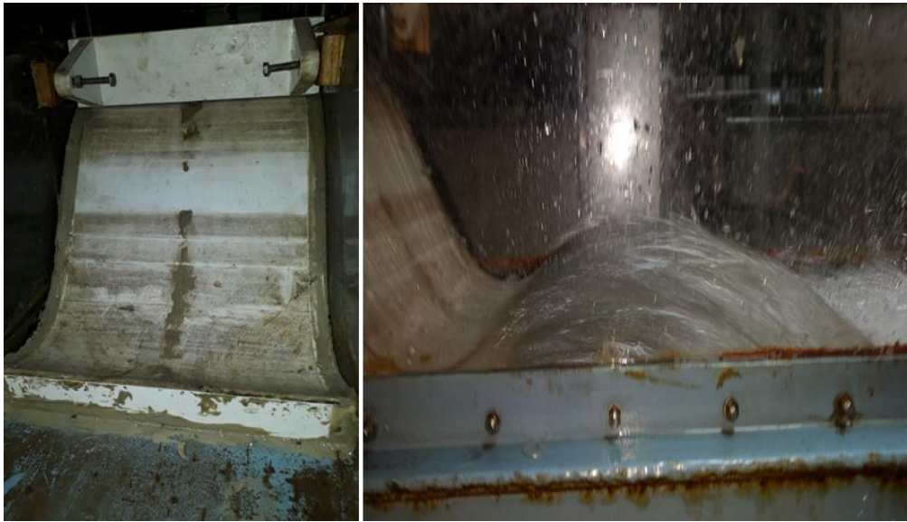
Figure.5. Downstream view of Conventional ski-jump bucket energy dissipator
