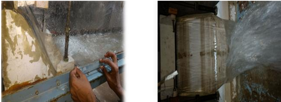
Figure.6. Downstream view of ski-jump bucket energy dissipator with Type I deflector
