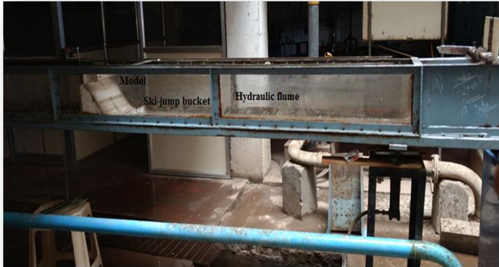
Figure.3. Conventional ski-jump bucket
