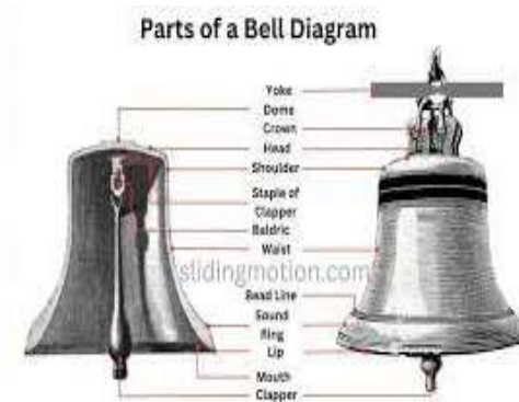
(Fig.18) Different parts of a bell 31
