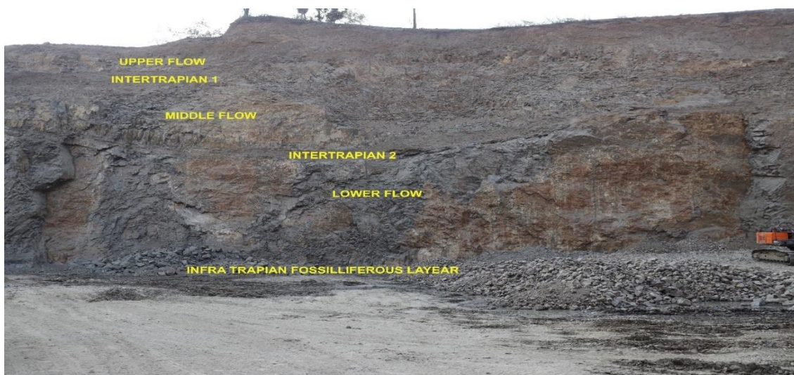
Fig No: 1. Field photograph of three basalt lava flows with intertrappean I & II and Infratrappean fossiliferous layer at the bottom in quarry cuttings observed in Sri Sivagowri stone quarry at Duddukuru.
