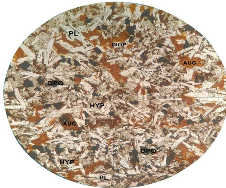
Fig : 7 . Micro Photograph Showing Sub-Ophitic and intergranular texture, with Plagioclase,Augite,Diopside,Hypersthene and Opaque in Basalt Sample at Duddukuru ( X 10 ) Under plane polarised light.
