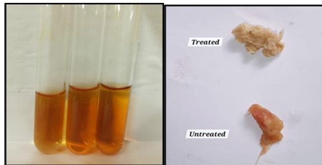
Fig. 7 (left) The Filtrate showing a red colouration after completion of the test. Fig. 8 (right) The treated and untreated sample subjected to Maule's test
