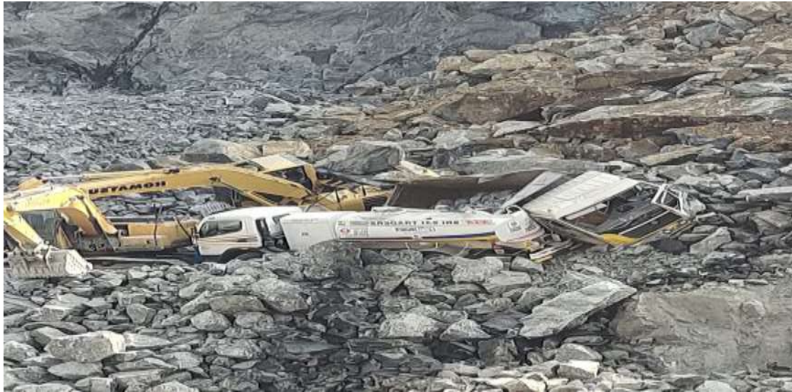
Chikkballapur accident due to fall of sides
