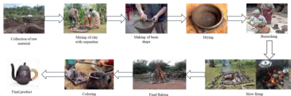
Fig. 4. Making process of black pottery
