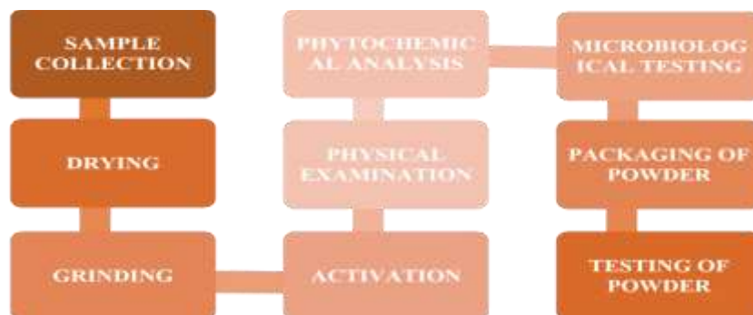
Figure 1. Flow chart depicting the preparation and evaluation of onion peel based effervescent water purifier powder.
