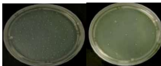
Figure 2. Reduction in bacterial colonies in water samples before and after treatment with effervescent water purifier powder.
