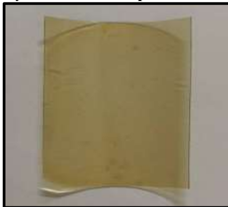
Figure 6 Carboxymethyl cellulose-based patch containing cinnamon crude extract and glycerol.
